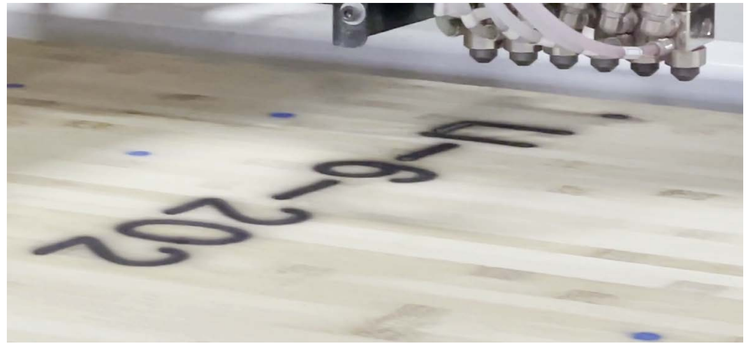
CUSTOMIZED ON PANEL MARKING Cimat machine instruction translates panel number, nail pattern and MEP placement map to Onsrud for direct panel printing
