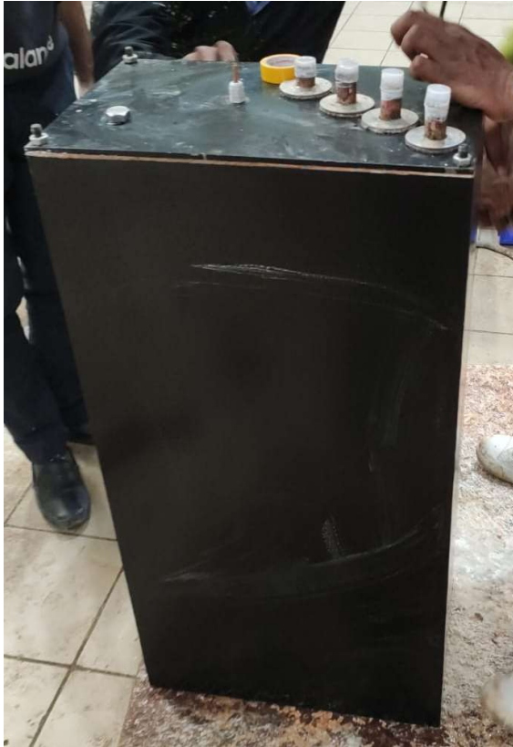
Insulated outer shell integrated with fin and tube heat exchanger
